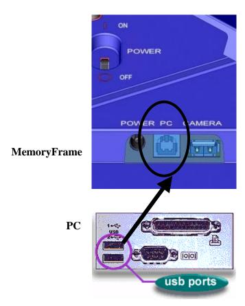
Figure 7 – Connecting a PC to MemoryFrame
